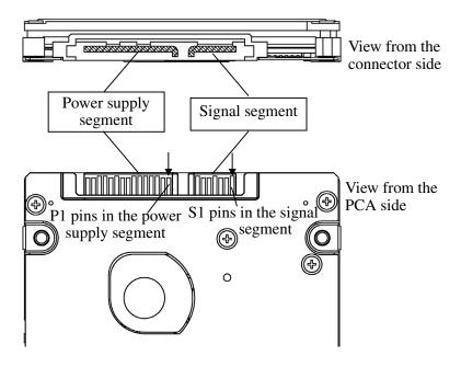
Figure 3.8 Power supply pins (CN1)
